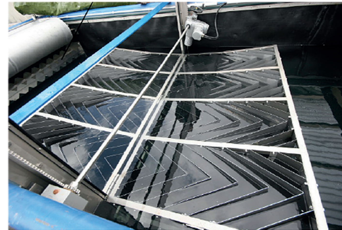
Figure 3: Experimental cross-flow lamella settler unit in cleaning position © UFT, Gebhard Weiß
